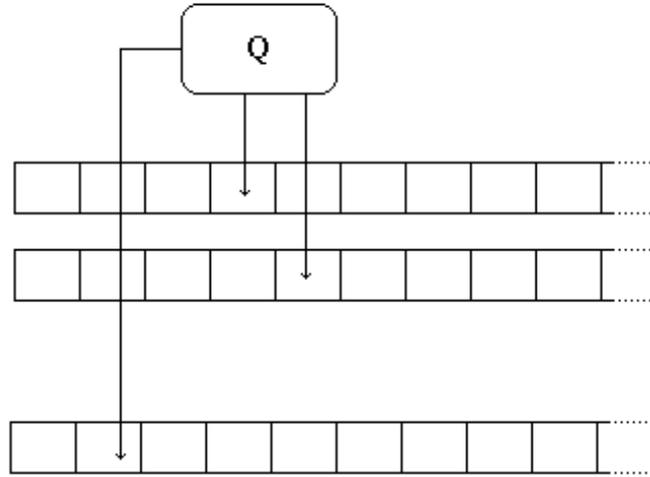
Figure 1: head and tapes of a Turing machine
